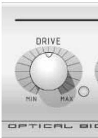
This needs to be set at a point where the processor receives the optimum level required for Big Bottom to work effectively. To find the optimum level, turn the control clockwise until the green L.E.D. at the right of the Drive control pulses on the bass peaks. Longer and brighter pulsation means a longer bass sustain is being created. You will find a range of settings that yields very musical and powerful bass.
