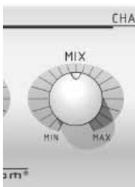
This control adjusts the amount of Big Bottom enhancement being added to the original signal. The lower the setting, the subtler the effect until there is no effect at all. The higher the setting, the more dramatic the effect.
